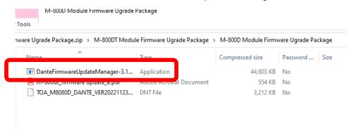
6. Run the Updater Manager and select the network on which the Dante Module is connected.
