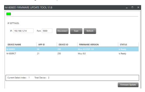
Upon completion, the M-8080D main unit will power cycle and will indicate the new firmware version (6.0) on the front panel. Congratulations! You are now ready to use the M-8080D Dante System. Make sure to use Version 2 of the M-8080D System Controller Software. Version 1 is no longer compatible with this Dante upgraded firmware.
